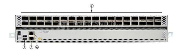
Note: (1)  $36\ 40$ -Gigabit QSFP+ ports (2) USB ports (3) Out-of-band management port (RJ- $45\ port$ ) (4) Console port (RJ2 $32\ port$ )
